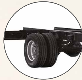
Rear-wheel drive with twin axle and air suspension on the drive axle
