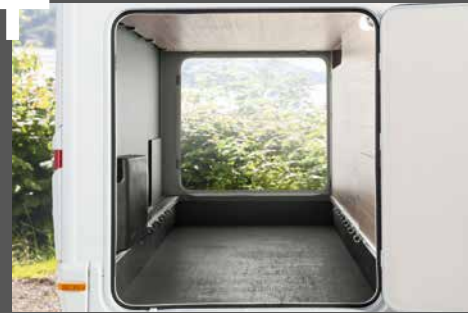
Large rear garages with access from both sides and new, smooth-running twist/quick-release latches
