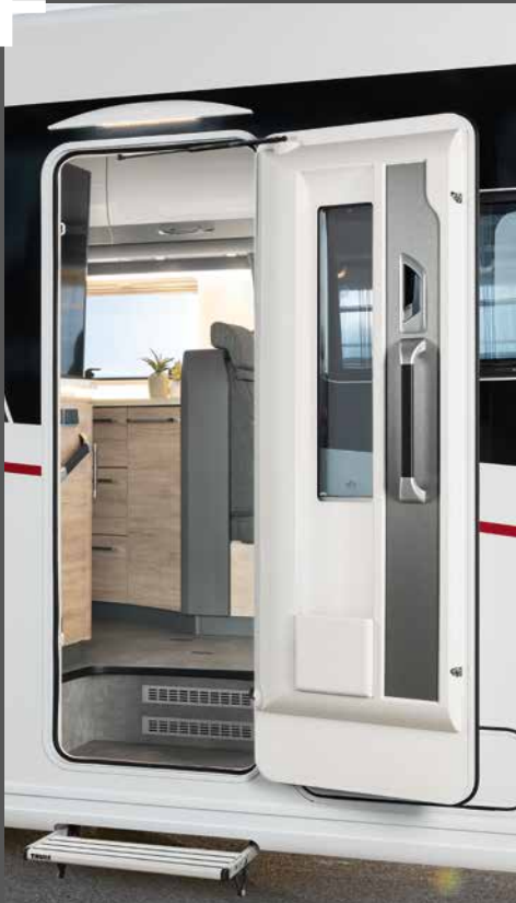
70 cm-wide door with window, central locking system and electric closing aid
